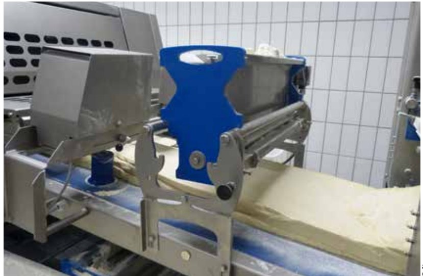
++ The dough pieces of the dough strand overlap one another, as can be seen at the start of the line
