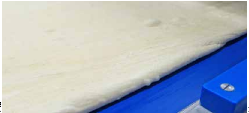
++ A quick reducer, cross roller and finishing station gently shape the dough sheet to the required dough sheet thickness. Fermentation bubbles are still visible in the dough
