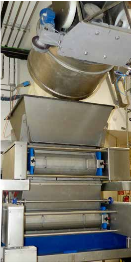
++ The start of the Crusto bread/bread roll plant, with a Double Chunker stress-free system to gently produce the dough strand
