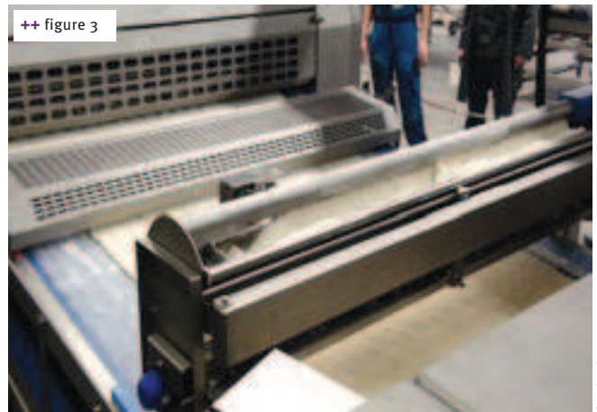
++ figure 3 The working width of the bread line is 1,600 mm
