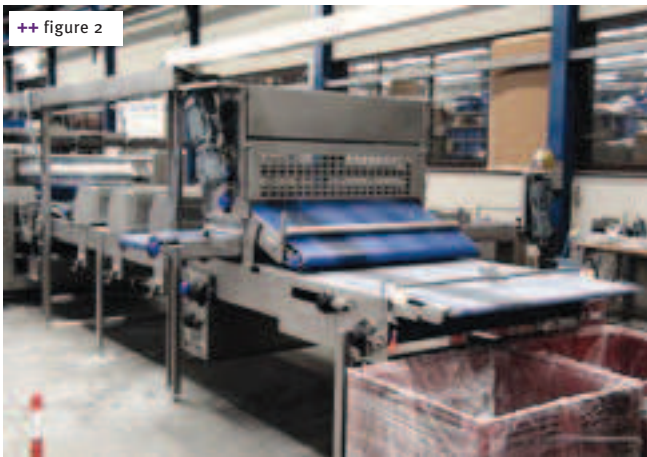
++ figure 2 The offtake station at the end of the plant ensures that the residual dough is removed
