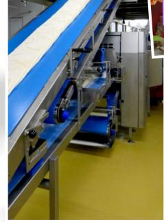
++ After lamination, the dough rests in an integrated cooling cabinet
