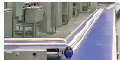
1. Inline Dough Recycling System: rework dough is directly transferred back into the pre-sheeter. This way no dough is lost during the production process.
