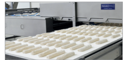
Our tray loading systems are able to precisely load the products onto the baking trays, peel boards, baking thins or transportation belts. We have developed several systems to provide a solution for every specific situation.
