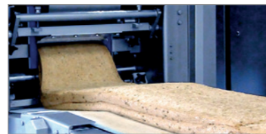
2. Bread dough pre-sheeters: generate stress-free dough sheets of any type with excellent weight control at the highest quality. The dough structure is untouched because of the dough friendly handling. We have several solutions available, depending on dough type.
