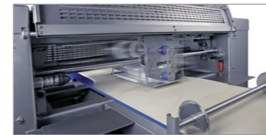
4. Cross roller: to compensate the one-sided reduction of the reduction stations and to adjust the dough sheet in thickness. The dough sheet will reduce in thickness and increase in width.
