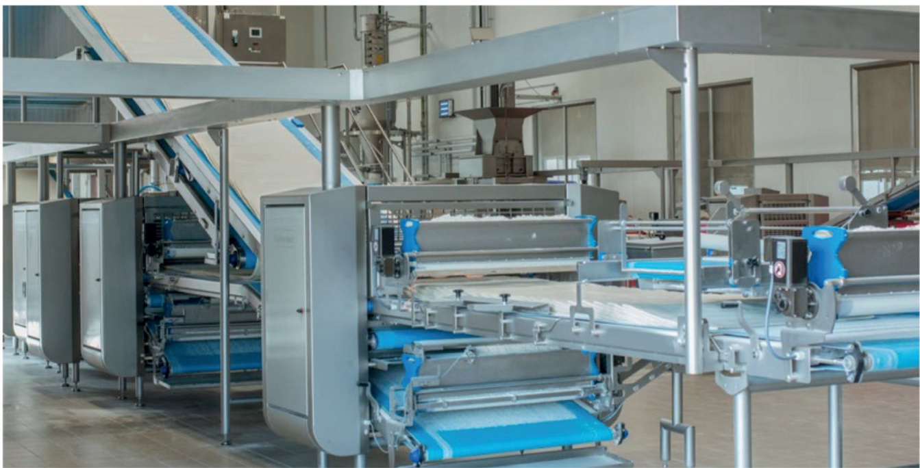
++ After reducing this final laminated dough sheet, it undergoes a cooling and resting period in Rademaker's Cooling and Resting system
