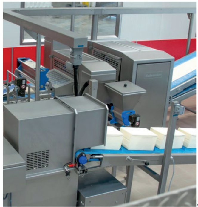
++ Rademaker's Fat pump processes butter blocks into a consistent butter layer
