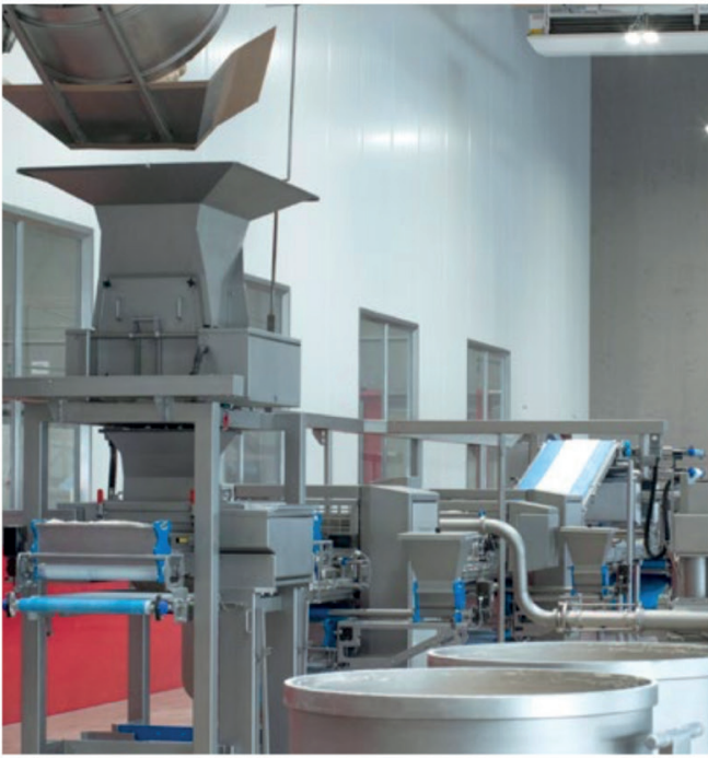
++ The dough batches are deposited into the a Chunker before it is processed by Rademaker's Low Stress Sheeting System
