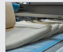
Rademaker developed three different laminating methods that can laminate the dough sheet up to 512 layers, depending on the line concept, dough type and capacities..
