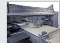
Cross-rolling to achieve the optimal working width of the dough sheet.
