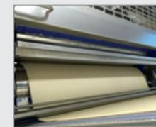
Reduction steps for a consistent, quality dough sheet (width and thickness).
