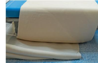
The belt with the dough sheet moves back and forth above the next conveying belt. This is an asymmetric lamination system suitable for soft dough with no restrictions regarding laminating width.
