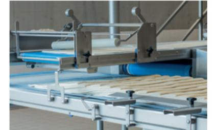
A guillotine cuts the dough sheet into regular rectangular sheets which are then stacked on top of each other. This flexible symmetric system lays even and uneven layers. Suitable for soft doughs with no restrictions regarding laminating width.
