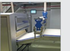
Final reduction step, the dough has now reached its final thickness.
