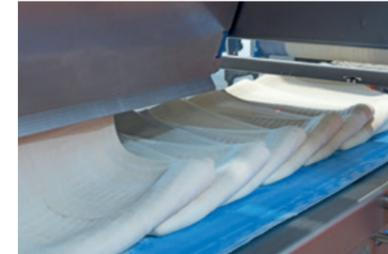
The dough sheet runs vertically between a guiding system that moves back and forth. This symmetric lamination method is unsuitable for soft dough and has a maximum lamination width of 600 mm.
