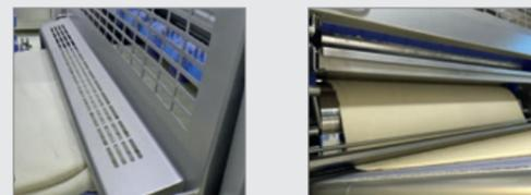
Reduction steps are applied for a consistent, quality dough sheet (width and thickness).
