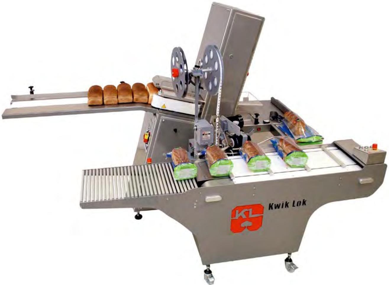
Semiautomatic Slicing and Packaging line for sliced and unsliced bread.
