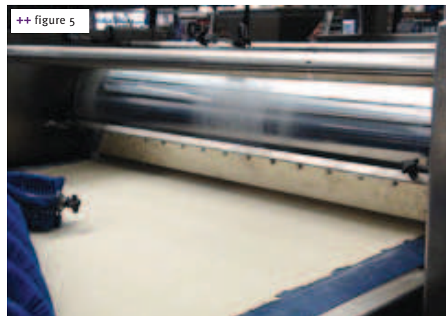
+ figure 5 The solid stainless steel rollers run very quietly
