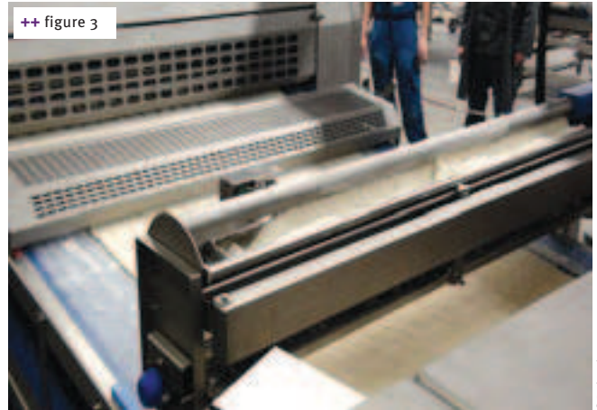
++ figure 3 The working width of the bread line is 1,600 mm
