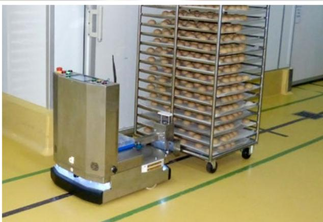
++ A robot carries rack trolleys within the production area
