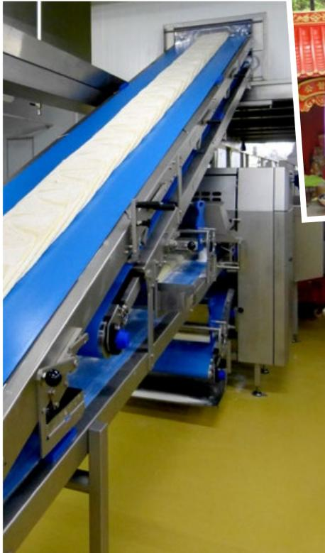
++ After lamination, the dough rests in an integrated cooling cabinet
