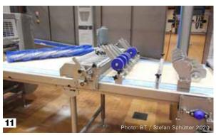
8 This feeder belt can feed a retractable sheeter for shortcrust pastry. Since shortcrust pastry is always very crumbly, it should only be rolled out as gently as possible.
