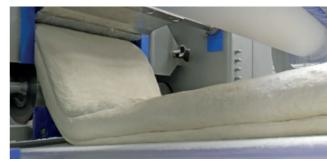
Elimination of falling heights: by minimizing the transportation height throughout the production line, it results in a stable and relaxed dough sheet.
