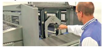
Efficient, error free operation and tool change-over is realized by applying Unique Fit Tooling. Because of the lightweight and more compact tooling, handling and detaching the tools is as easy as possible and can be done by one person. No other devices are needed to help the operator change the tools.
