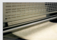
5. Reduction station: the thickness of the dough sheet is reduced while passing through the rollers.
