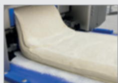
1. Dough pre sheeters: generate stress-free dough sheets of any type with excellent weight control at the highest quality. The dough structure is untouched because of the dough friendly handling.
