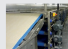
7. Proofing: the dough sheet or products can be in-line proofed, depending on the type of products and production process.
