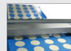
8. Rework station: the rework dough is transported back to the pre-sheeter or mixer. This brings our Flatbread line to a highly effective and cost saving level.
