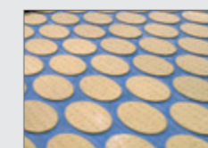
9. Topping station: a module for seeding the baked products, e.g. with sesame or other seeds, can also be integrated into the plant
