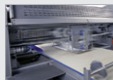
4. Cross roller: to compensate the one-sided reduction of the reduction stations and to adjust the dough sheet in thickness. The dough sheet will reduce in thickness and increase in width.
