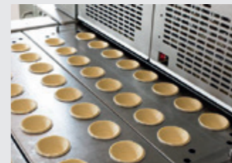
4 The dough billets are pressed without rework.
