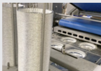
2 The cup denester ensures that the foil is correctly placed.
