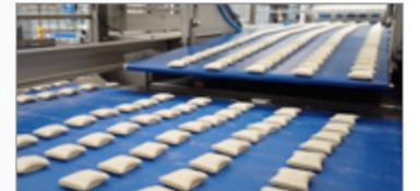
Our Tray loading systems are able to precisely load the products onto the baking trays, peel boards, baking thins or transportation belts. We have developed several systems to provide a solution for every specific situation.
